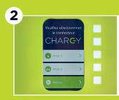
Select your connector (connector 1 or connector 2) by pressing the button next to the display.
